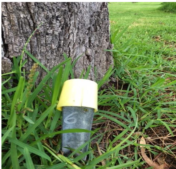
Figure 3: Example subsidence monitoring point with safety cap.
